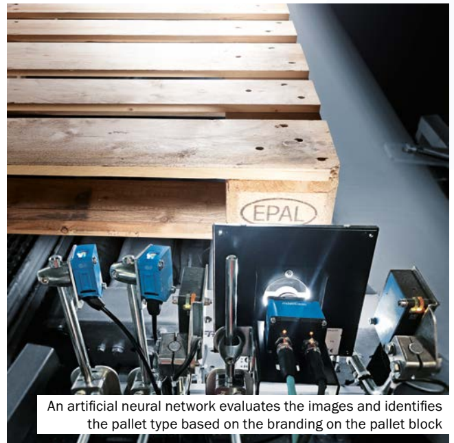
PACS can be mounted at any position along the conveyor system and captures images of the pallet blocks from two sides
